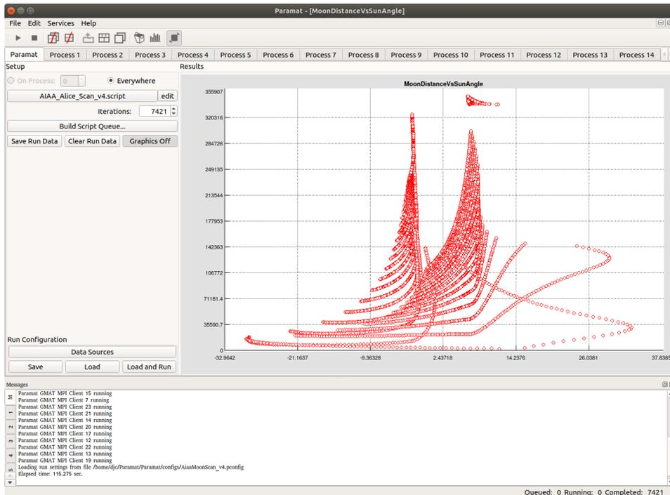
**Figure 3. Lunar Periapsis Distance vs Solar Beta Angle for 7421 trajectories**
