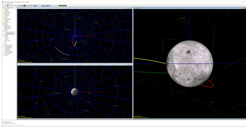
**Figure 2. Starting Conditions for the Flyby Search. The upper left view shows the inertial trajectory as seen from above the Earth. The lower left view shows the Moon from above. The right view looks at the trajectory along the Sun-to-Moon vector.**
