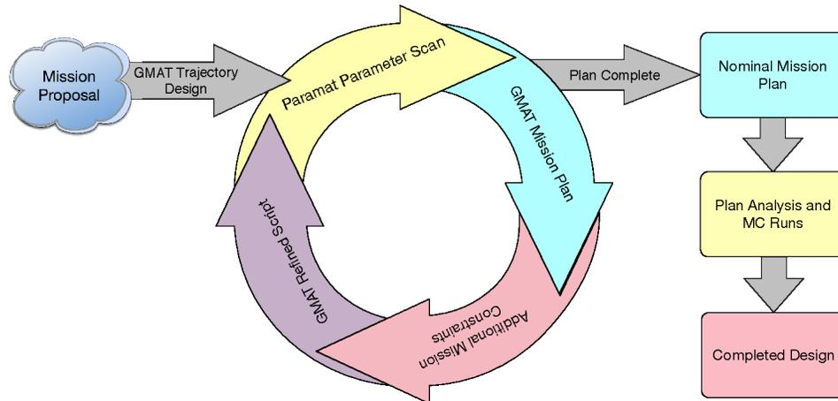
**Figure 1. The GMAT/Paramat Mission Design Workflow**
