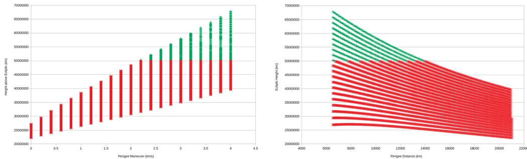
**Figure 8. The Trade-off Between Earth Flyby Distance and Maneuver Delta-V. The points in green achieve the mission goal of a minimum 50,000,000 km above the ecliptic.**
